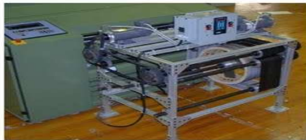
Figure 4. Web divider with servomotors and digital control
